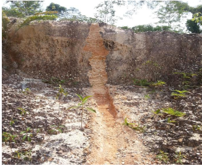
Foto 1 : Location alluvial deposit at the site IUP Aurum Persada PT Equator and trench sampling test methods
