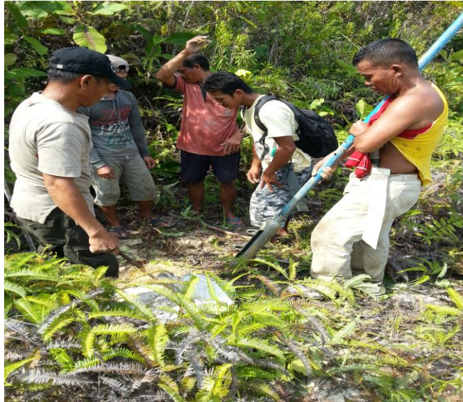
Foto 3 : Activities prior to the implementation of a hand drill sampling, sampling depth capacity with such a device up to 8.5 m
